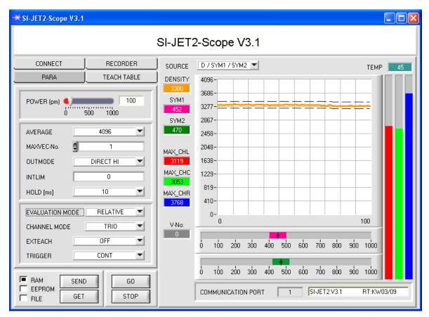
In EVALUATION MODE RELATIVE all three channels CH\_L, CH\_C, and CH\_R are standardised in relation to their respective maximum values during the last 60 seconds. These standardised values are then used for determining density, symmetry 1, and symmetry 2. The advantage of this evaluation mode is that the standardisation to the respective maximum value to a large extent compensates possible dirtying of the sensor.
